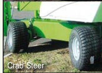
The extra manoeuvrability available from the 4 wheel steer option coupled with the special "Turf Tyres" make the SD210 ideal for working on sensitive surfaces such as grass.
